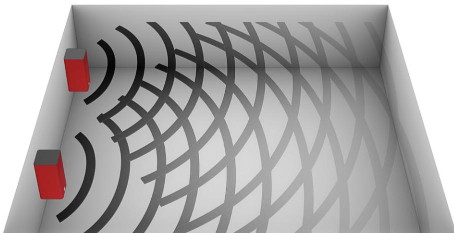
The wide dispersion characteristics also add to the flexibility of the KUBIK FREE system, making it possible to hang or place it flush against the wall, or position it on a table in the middle of a room. Placement of the KUBIKs close to or against a wall is however recommended for optimum bass reproduction.
